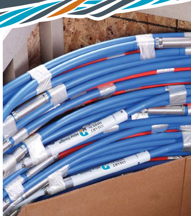
MPBXs can be used to monitor movements around large underground caverns
